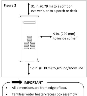
Tankless water heater/recess box assembly are zero inches to all surfaces of the recess box. A 24 in. (610 mm) clearance to combustibles and non-combustibles must be maintained from the front of the unit for servicing.
