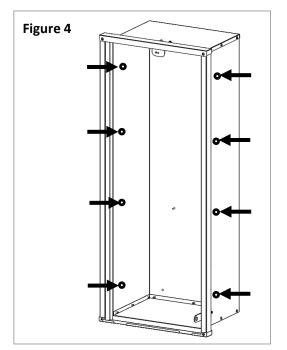
2. Using the supplied piping template (last page in this document), drill 4 holes in the bottom of the recess box to accommodate the hot water, cold water, gas and electric lines. The pressure relief valve (PRV) location is not identified on the template.
